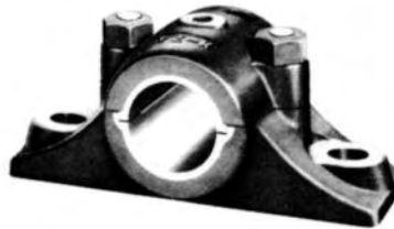
Type K Split Babbitted Bearing. Gibs are molded in the Babbitt lining. Supplied babbitted only with two cap bolts and two base mounting holes.
