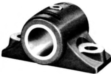
Type J Solid Bearing. Supplied with two base mounting holes only. Can be babbitted or bronze bushed.
