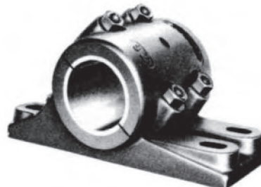
Type L Split 40 Angle with hollow dowel pins to align the cap with the base plus relieve side pressure. Either babbitt liner or split bronze bushing available.
