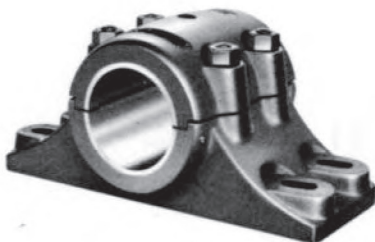
Type MG Split with Machined Gibs in the iron base and cap to relieve side pressure. Supplied four bolt with Babbitt liner or split bronze bushing.
