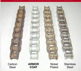
After 14 days of exposure to 5% salt spray solution.
